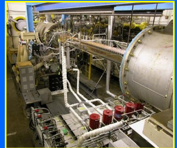
Direct-Connect Supersonic Combustion Test Facility (DCSCTF) Flight Mach Enthalpy: 4.5 - 7
