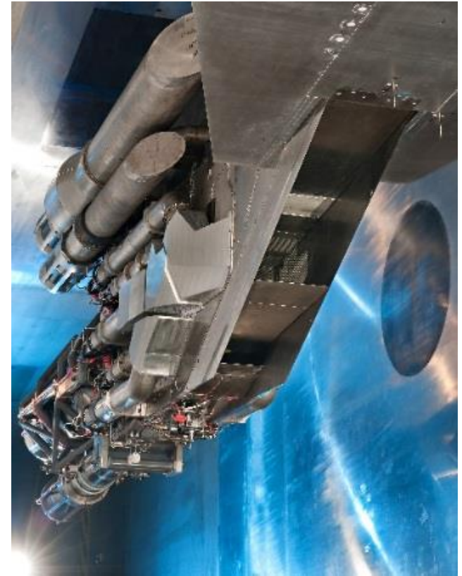
Combined Cycle Engine Testing in GRC 10x10
