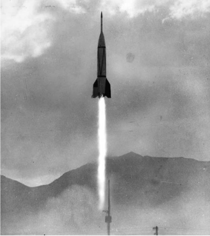
Fig. 1.1 V-2/WAC Corporal liftoff on 24 Feb. 1949, the first object of human origin to achieve hypersonic flight (National Air and Space Museum).
