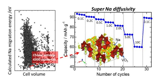
A high-throughput computation for Na migration energies is conducted for about 4,300 compounds in the inorganic crystal structure database, which the compound indeed exhibited excellent high-rate performance and cyclic durability; in detail, the compound exhibits stable 10C cycling, which
