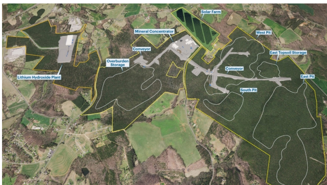
Figure 5 – Site plan for the planned permit area of the Phase 1 30,000 t/y Carolina Lithium operations
