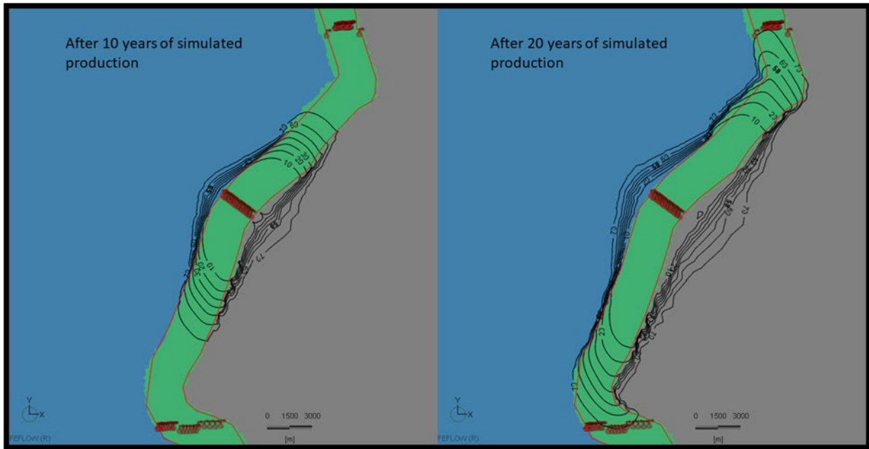
Figure 16-11. Simulated lithium concentration (mg/L) after 10 and 20 years based on an average annual production rate of 128,800 m 3 /day.
