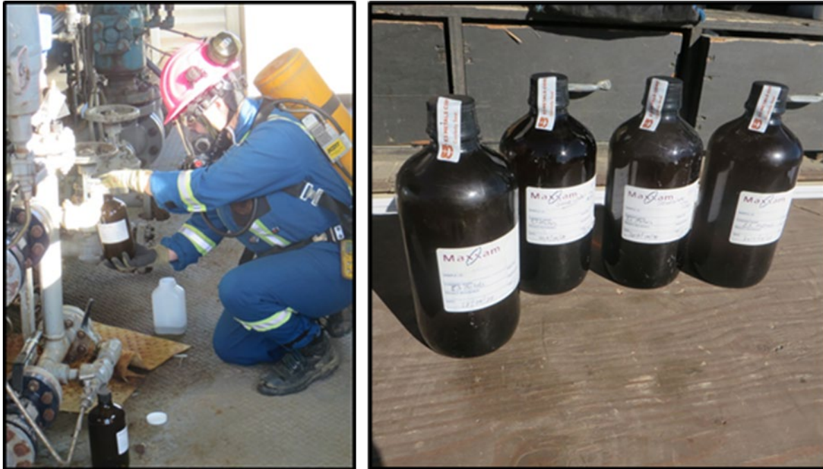
Figure 9-3. Sample collection at test separator. Left: Maxxam employee collecting sample from test separator access port. Right: Sealed well samples.
