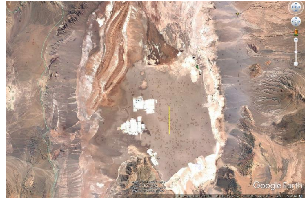
Image: Satellite image of the Salar de Atacama. The brine extraction and evaporation operations of SQM can be seen in the centre of the 'salar', with Albemarle's operations fringing the south peninsular of the 'salar'. The yellow bar represents a distance of ~10km. Source: Google Earth.
