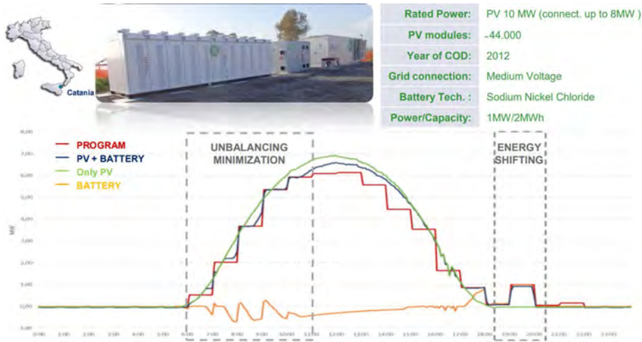
Figure 3.5: Solar Photovoltaic Installation with a Storage System
