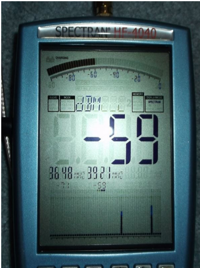
Figure 1. Typical Spectran HF-4040 reading taken in summer 2016. 3648 MHz at -71dbm and 3921 MHz at -59 dbm. There are very few users in this frequency range – so it is easy to identify. Scans were typically done by sweeping between 3500 MHz and 4000 MHz, but could be narrower, once the range is known.
