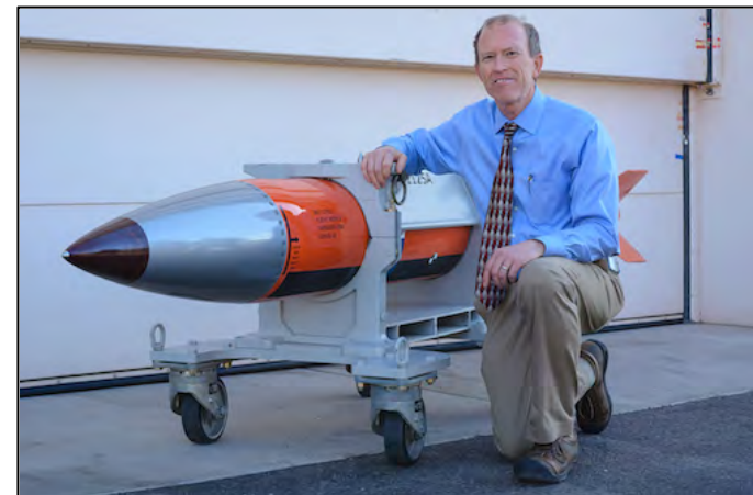
(Above) The most powerful U.S. conventional bomb – the GBU-43/B Massive Ordnance Air Blast (MOAB) – has an explosive yield of approximately 0.011 kt TNT, roughly 30 times less than the lowest yield setting (0.3 kt) on the B61 nuclear bomb (below). The B61-12 weighs 850 lbs (385 kg), nearly thirty times less than the MOAB's 22,600 lbs (10,300 kg).
