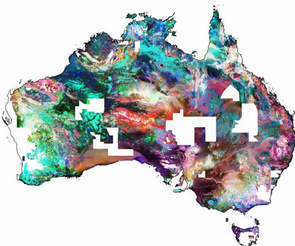
FIG. 3. Ternary image (K-red, eU-blue, eTh-green) of Australia derived from the new levelled National Radioelement Database.
