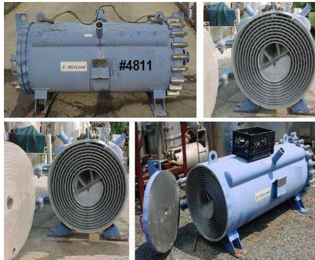
FIG. 6. Secondary heat exchanger.
