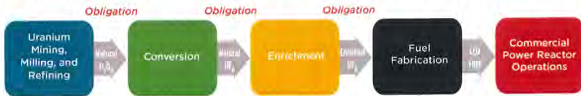
Figure 4. Commercial Production of LEU Fuel
