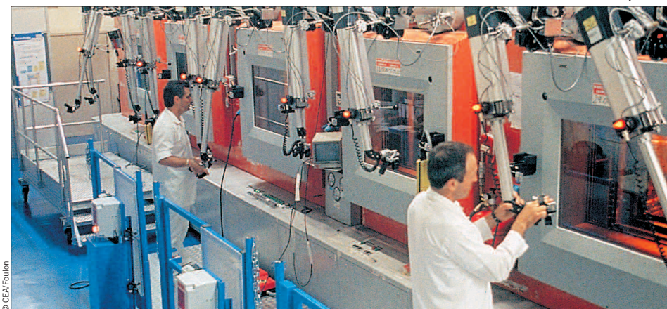
Shielded vitrification line for fission products.
