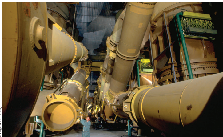
Diffusers at Eurodif's Georges Besse plant.
