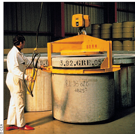
Conditioning waste in a concrete matrix.
