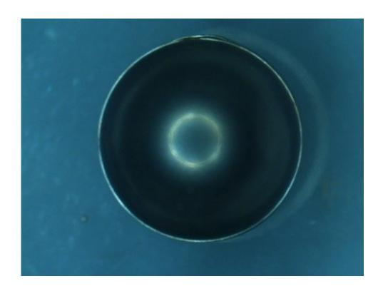
3.6mm-diameter, 40um-thick, 20mg B-filled diamond shell. Credit: R. Moyer, University of California, San Diego.
