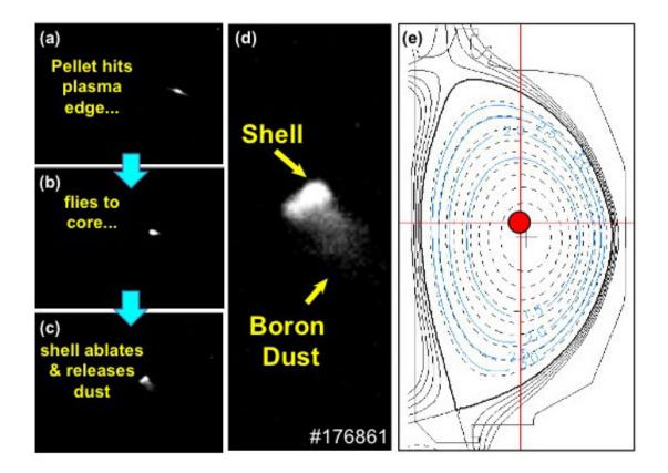
Visible imaging of (a) shell pellet hitting low-field-side boundary of plasma, (b) continuing through plasma toward core, (c) ablating and releasing boron dust in core. (d) Expanded view of (c), highlighting shell and dust. (e) Plasma cross-section with red dot indicating pellet location at time of dust release in (c). Injection velocity 230 m/s. Credit: R. Moyer, University of California, San Diego.
