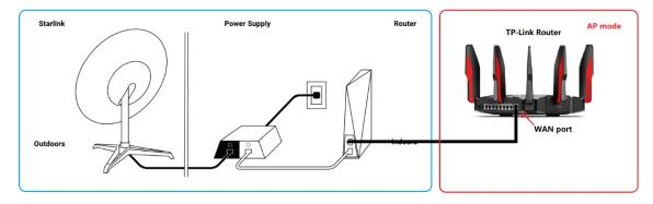
On this network topology, please connect the TP-Link router to the AUX port of the Gen-1 Starlink Router. To avoid double NAT, it is suggested to change the TP-Link router into Access Point mode.
