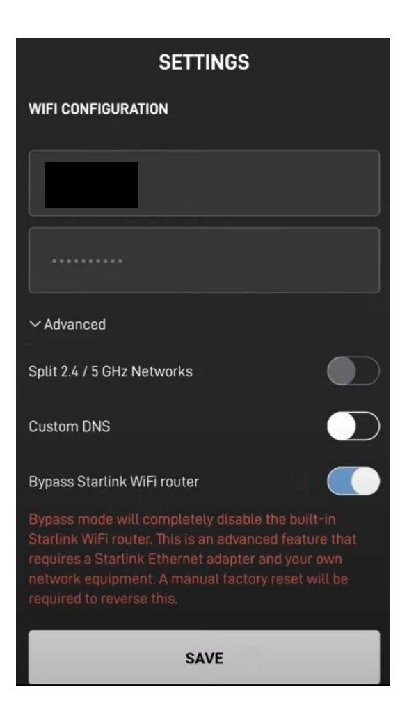
2. Leave Bypass mode disabled on Starlink APP, then set up the TP-Link router in Access Point mode.
