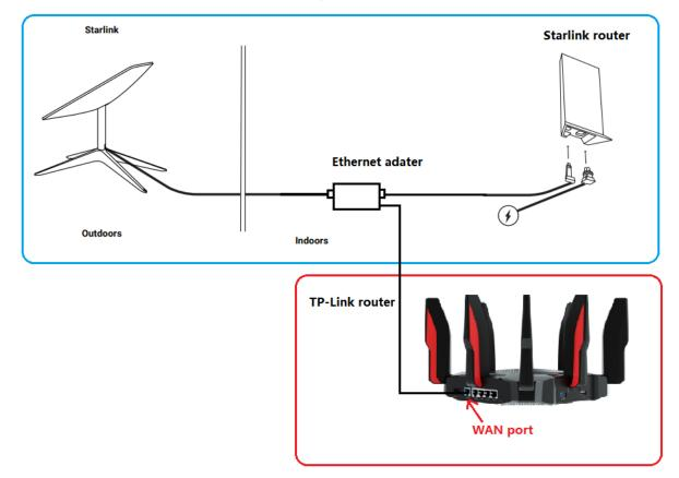
• Connect the TP-Link router together with the Gen-2 Starlink router
