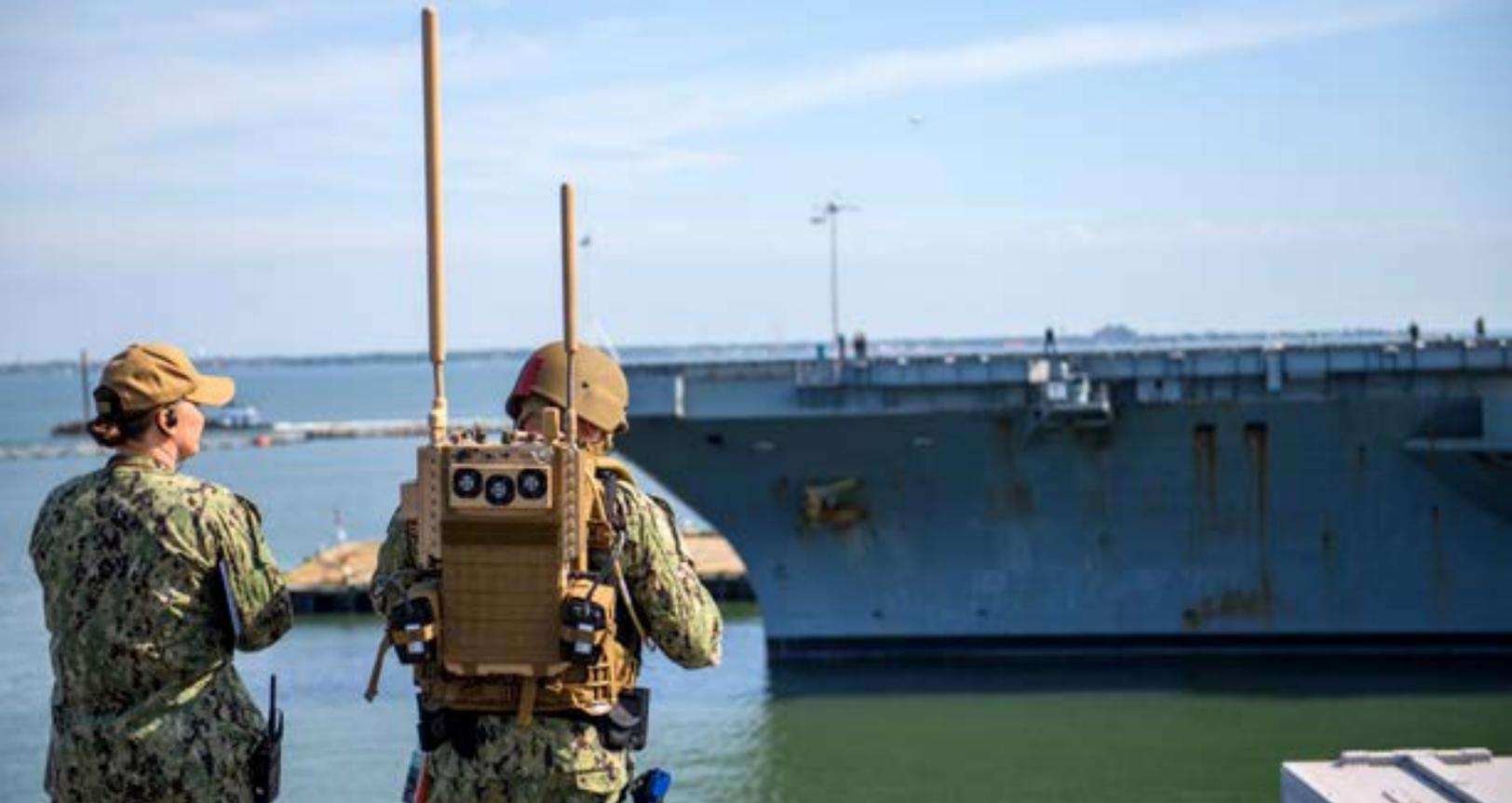
Photo: Master-at-Arms 2nd Class Leonard Gallegos, from Reno, Nevada, operates Drone Restricted Access using Known Electronic Warfare (DRAKE) module in a counter Unmanned Ariel System (UAS) security drill aboard the Nimitz-class aircraft carrier USS Dwight D. Eisenhower (CVN 69). Credit: Mass Communication Specialist 3rd Class Zachary Elmore/ US Navy
