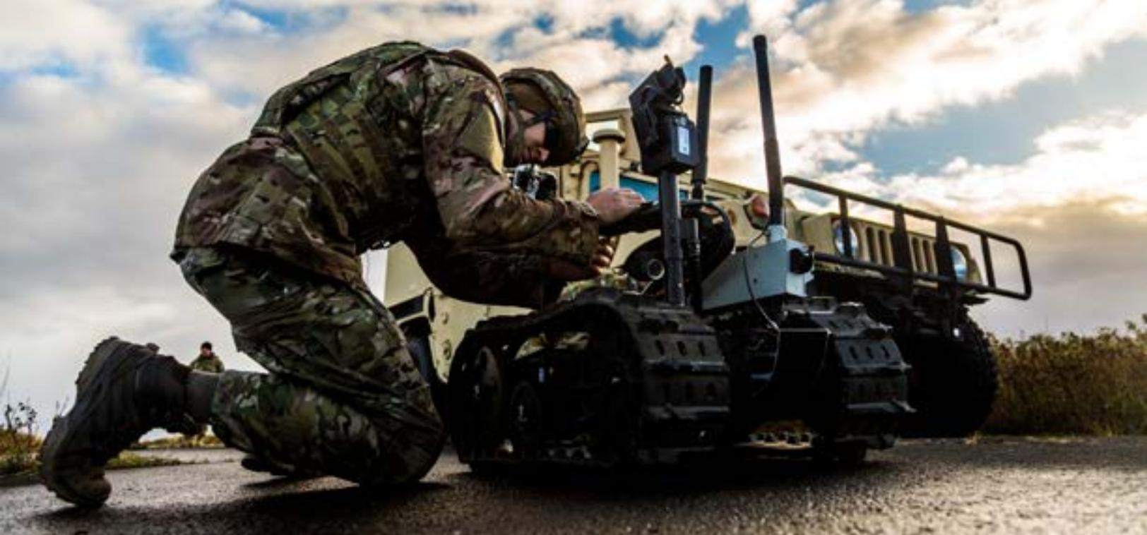
Photo: A US Air Force Explosive Ordnance Disposal (EOD) technician prepares a Mk. II Talon bomb disposal robot for work during exercise Northern Challenge. Credit: NATO
