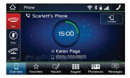
To end the call, press the **PHONE ON HOOK BUTTON** or touch the red "End" soft key.
