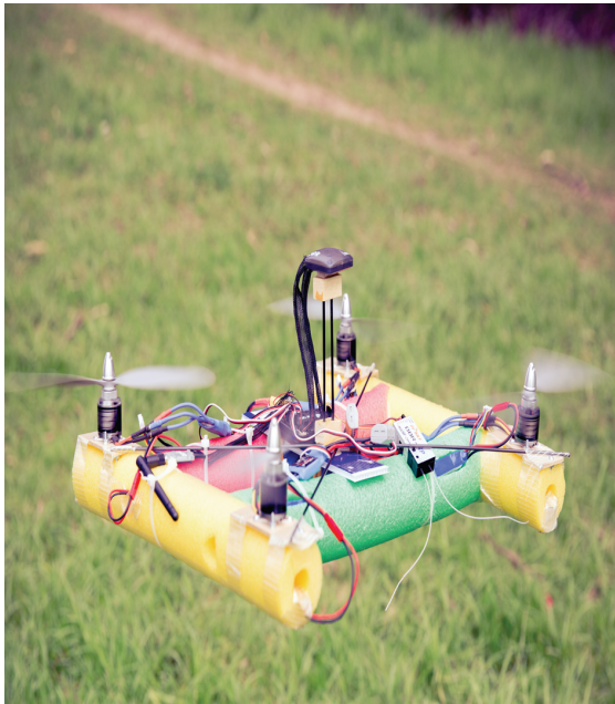
Figure 10-1 Structural supports for this drone are made from styrofoam pool noodles
