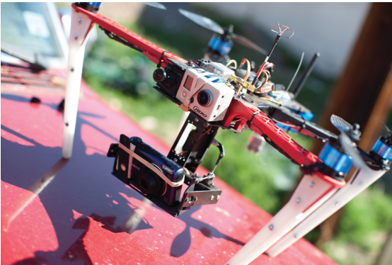
Figure 6-5 The aircraft is crooked but the camera is level, controlled by a brushless gimbal
