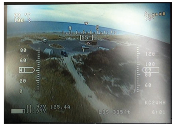
Figure 8-1 A true heads-up display: video from drone, overlaid with flight information
