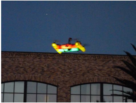
Figure 10-2 Pool noodle copter lit up with internal LEDs
