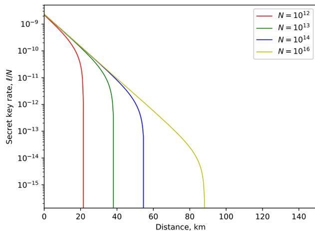
**Figure 4.** Illustration of the secret key rate (in logarithmic scale) in terms of the transmission distance (km), for a fixed amount of signals  $N = 10^{12}$ ,  $N = 10^{13}$ ,  $N = 10^{14}$  and  $N = 10^{16}$ .
