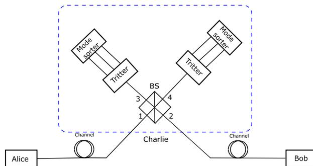
**Figure 2.** The generic measurement set up for our proposed MDI-QKD. Alice and Bob start by preparing the biphoton states from two mutually unbiased bases and send them through the unsecured channel to Charlie. Charlie allows the states to interfere in the symmetric beam-splitter (BS) upon receiving the states. The photons are directed towards the tritter and eventually detected in the Brown Twiss scheme (mode sorter).
