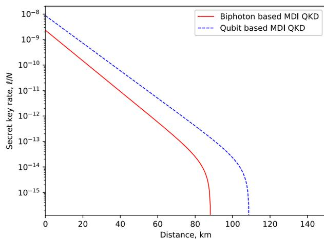
**Figure 5.** Illustration of the secret key rate (in logarithmic scale) in terms of the transmission distance (km) for our proposed biphoton MDI-QKD and the qubit-based MDI-QKD proposed in Ref.<sup>55</sup> for a fixed amount of signals  $N = 10^{16}$ .
