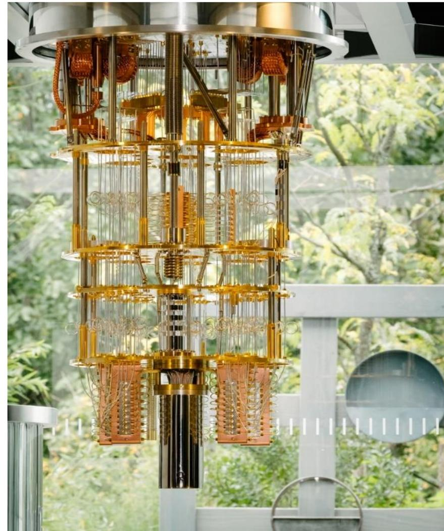
IBM 53-qubit superconductor-based quantum computer
