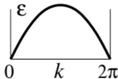
$$H_{\text{fermion}}^{\text{critical}} = \sum_{k \in [-2\pi, 2\pi]} 2i e^{i\frac{1}{2}k} \psi_{-k} \psi_k = \sum_{k \in [0, 2\pi]} \epsilon(k) \psi_k^\dagger \psi_k, \quad \epsilon(k) = 4 \left| \sin \frac{k}{2} \right|.$$
