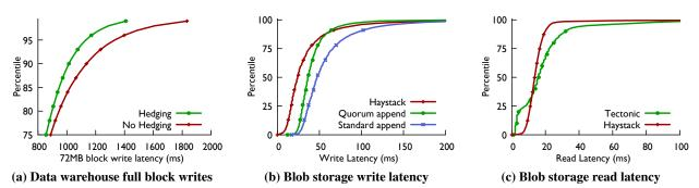
Figure 3: Tail latency optimizations in Tectonic. (a) shows the improvement in data warehouse tail latency from hedged quorum writes (72MB blocks) in a test cluster with ~80% load. (b) and (c) show Tectonic blob storage write latency (with and without quorum appends) and read latency compared to Haystack.
