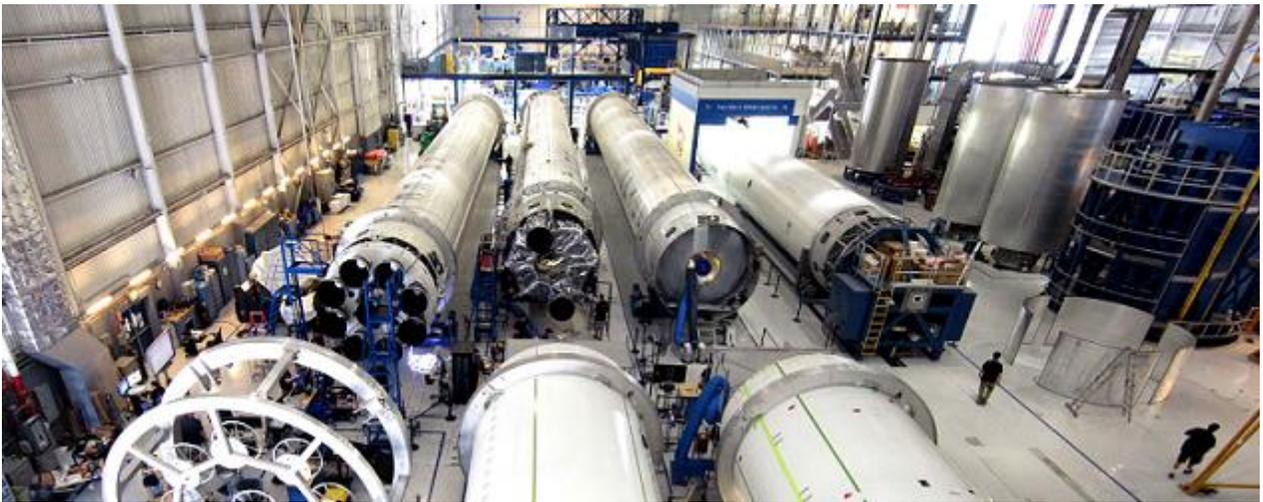
SpaceX engineers are busily processing the Falcon 9 fleet for a salvo of missions that will mark the company's return for the CRS-7 failure. The replacement of helium bottle support struts – one of which is suspected to have caused the CRS-7 mishap in June – is being conducted alongside additional changes, as SpaceX prepare for up to four launches by the end of the year, starting with a preliminary RTF date in November.
