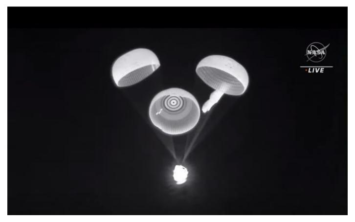
This still from NASA's Crew-2 landing webcast on Nov. 8, 2021 shows the delayed opening of one of four parachutes on SpaceX's returning Dragon capsule carrying astronauts home from the International Space Station. (Image credit: NASA TV)
