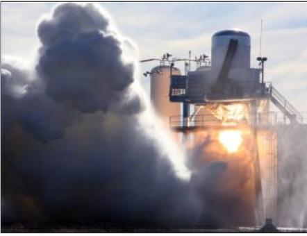
The second stage was test fired in a second, smaller McGregor test stand for 40 seconds during November. On January 2010, the Falcon 9 second stage completed a full duration mission firing, its Merlin Vacuum engine producing 41.96 ton thrust for 329 seconds. The stage was shipped to the Cape, where it arrived on January 29, 2010. There, it joined the first stage in the new SpaceX SLC 40 horizontal integration hanger.
