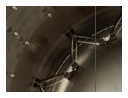
There were also <u>notes (L2)</u> about interest in the rods that <u>support</u> the helium <u>bottles</u> inside the LOX tank in the <u>second</u> stage.
