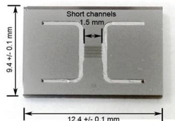
Optical image of the Microchannel Diffusion device.
