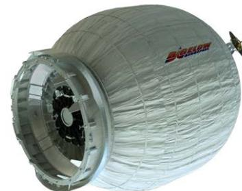
The Bigelow Expandable Activity Module (BEAM) is an experimental expandable capsule that attaches to the space station.
