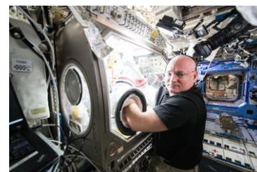
Astronaut Scott Kelly is photographed working with the Microgravity Sciences Glovebox (MSG) during a separate CASIS Rodent Research session using the Bone Densitometer
