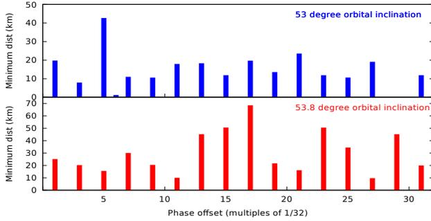
**Figure 1: Minimum passing distance vs phase offsets**
