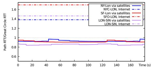
Figure 8: Latency using laser and RF co-routing.
