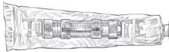
A toothpaste tube used as concealment for the CIA STINGER, a small .22-caliber single-shot firing device.
