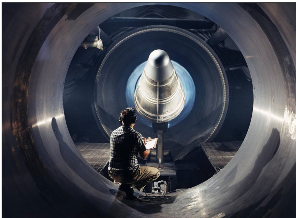
Figure 6: NASA Langley's 8-Foot High Temperature Tunnel Testing a Large-scale Cone Aerothermodynamic Test Article
