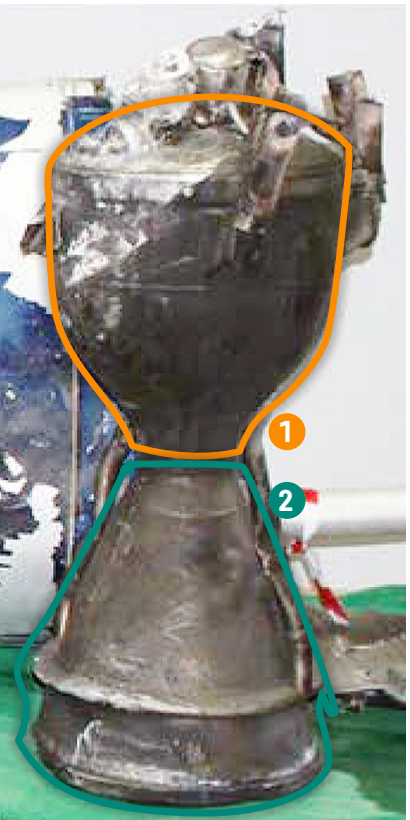
Burkan/Qiam engine debris recovered after a 4 November 2017 Houthi attack against King Khalid International Airport in Saudi Arabia Photos: DVIDS
