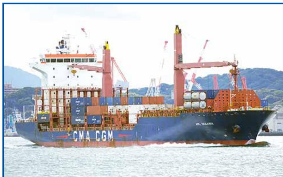
**APL OCEANIA UNDER WAY OFF JAPAN:** The APL Oceania is a geared container ship calling in the northern Marianas Islands and Japan. The ship along with its sistership the APL Islander serve as an important feeder link for larger liner vessels. She is crewed on deck by SUP sailors.
